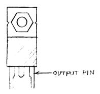
The voltage should be between +4.8v and +5.2v at Ul & U37. If the regulator doesn't meet this test, then check the board for shorts or errors.
