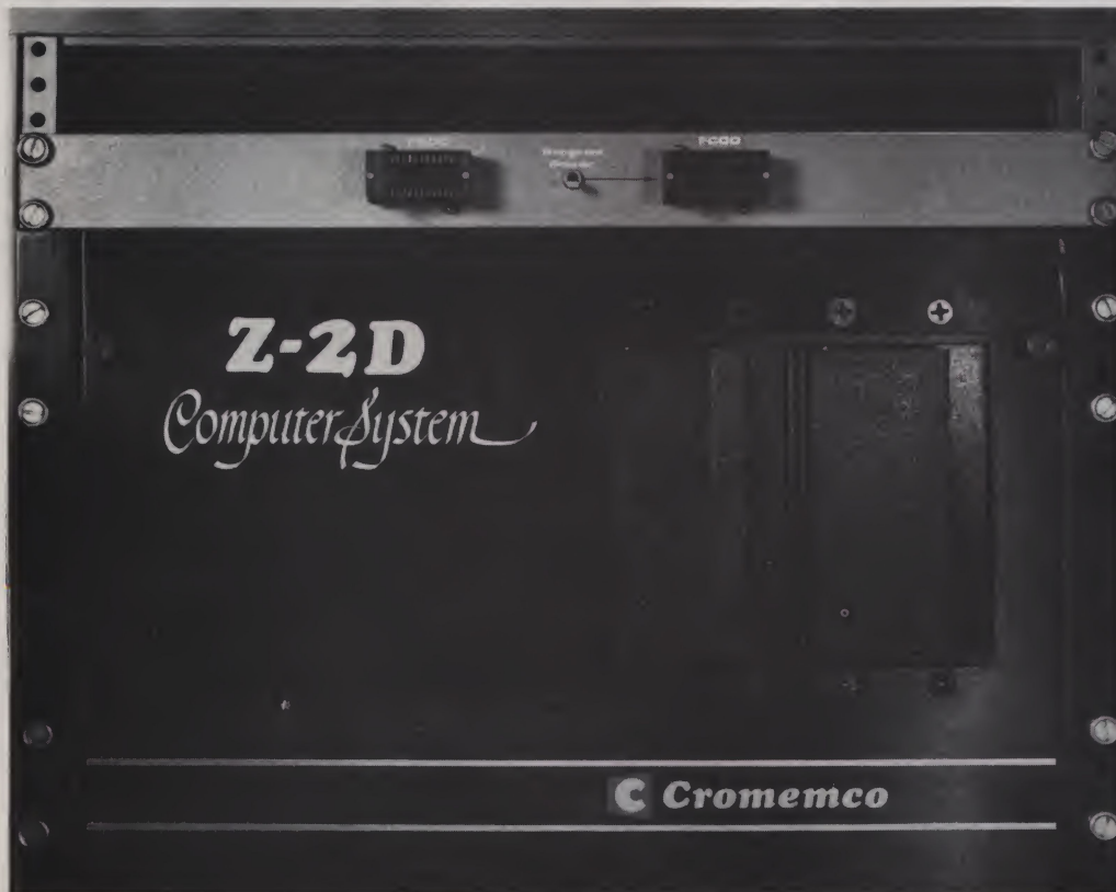
Photo 1. Front panel view of the Remote Programming Panel for the Cromemco Bytesaver, married to the author's Z-2D. The socket on the left, addressed at F800, is read-only; the one on the right, at FC00, is for programming. The metal switch handle is a useful ground point for the elimination of bodily static charge prior to insertion or removal of a 2708.
