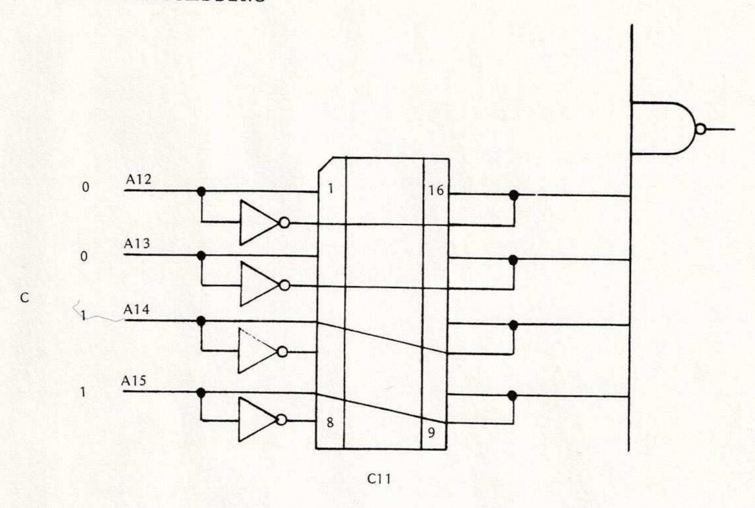
The board address select jumper location is Cll. It permits any one of the 16 possible 4K blocks of memory space to be jumpered to form the board enable.
