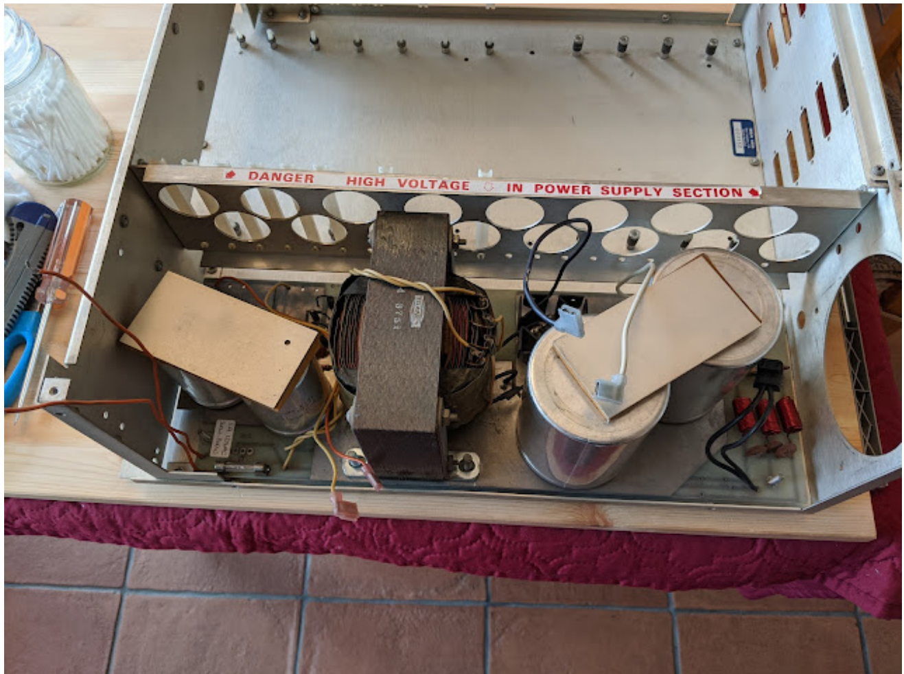
PSU in place on bolts.
