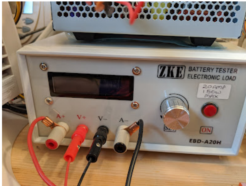
ZKE EBD-A20H Electronic Load Tester. 20Amp, 30v max.
