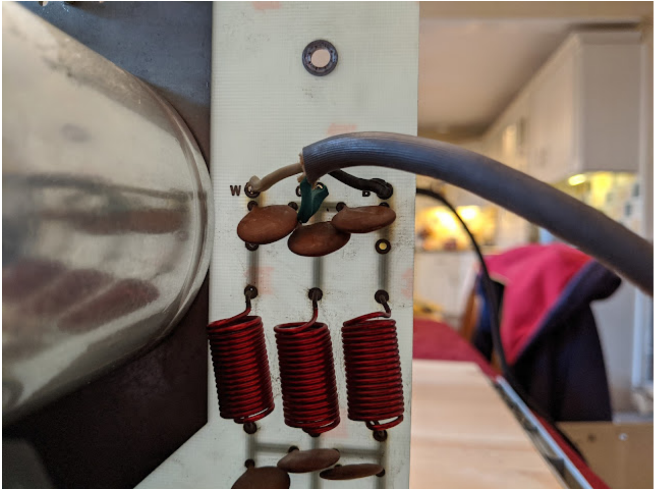
Mains cable fed through from the top side of the PSU pcb.
