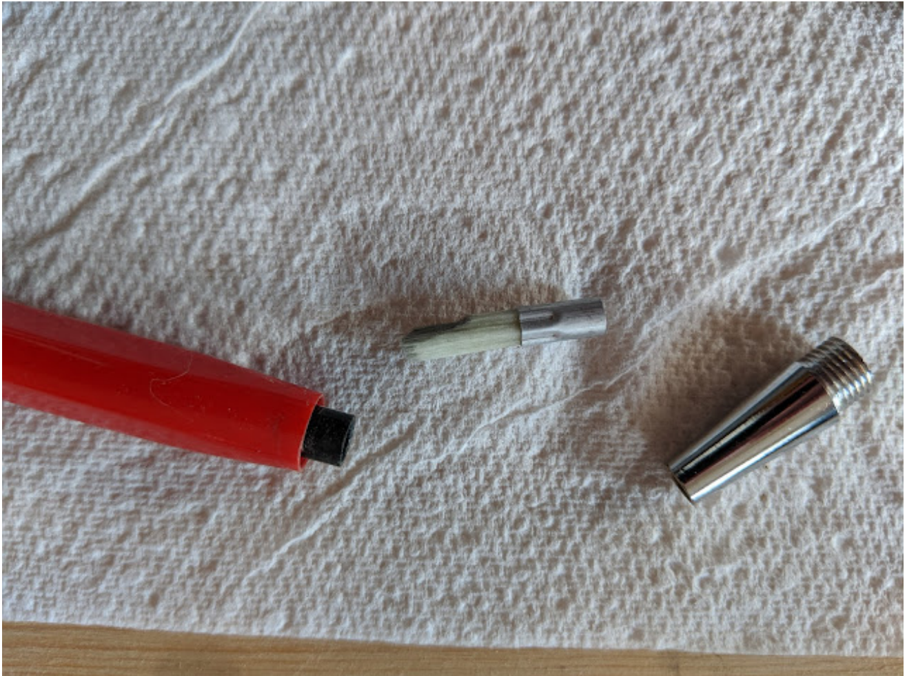
Effect of rubbing tip sideways along contacts.
