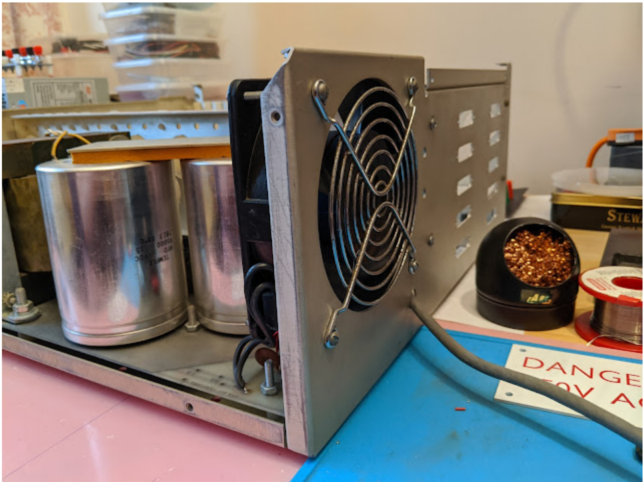
Guard in place over fan blades.
