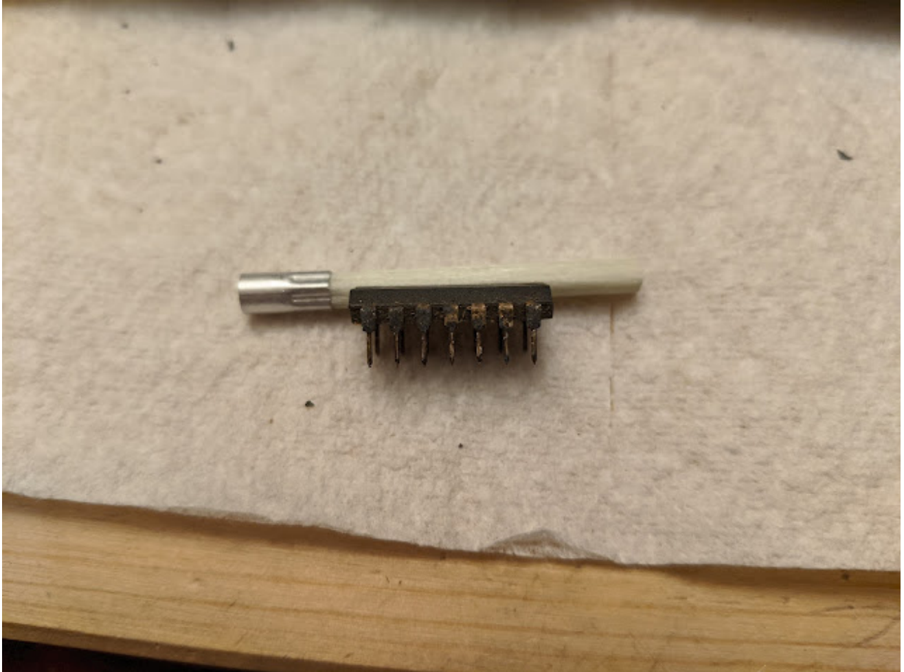
Fibre pen used for cleaning legs of ICs.
