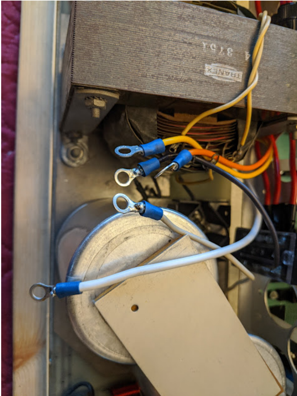
DC cables crimped and soldered.
