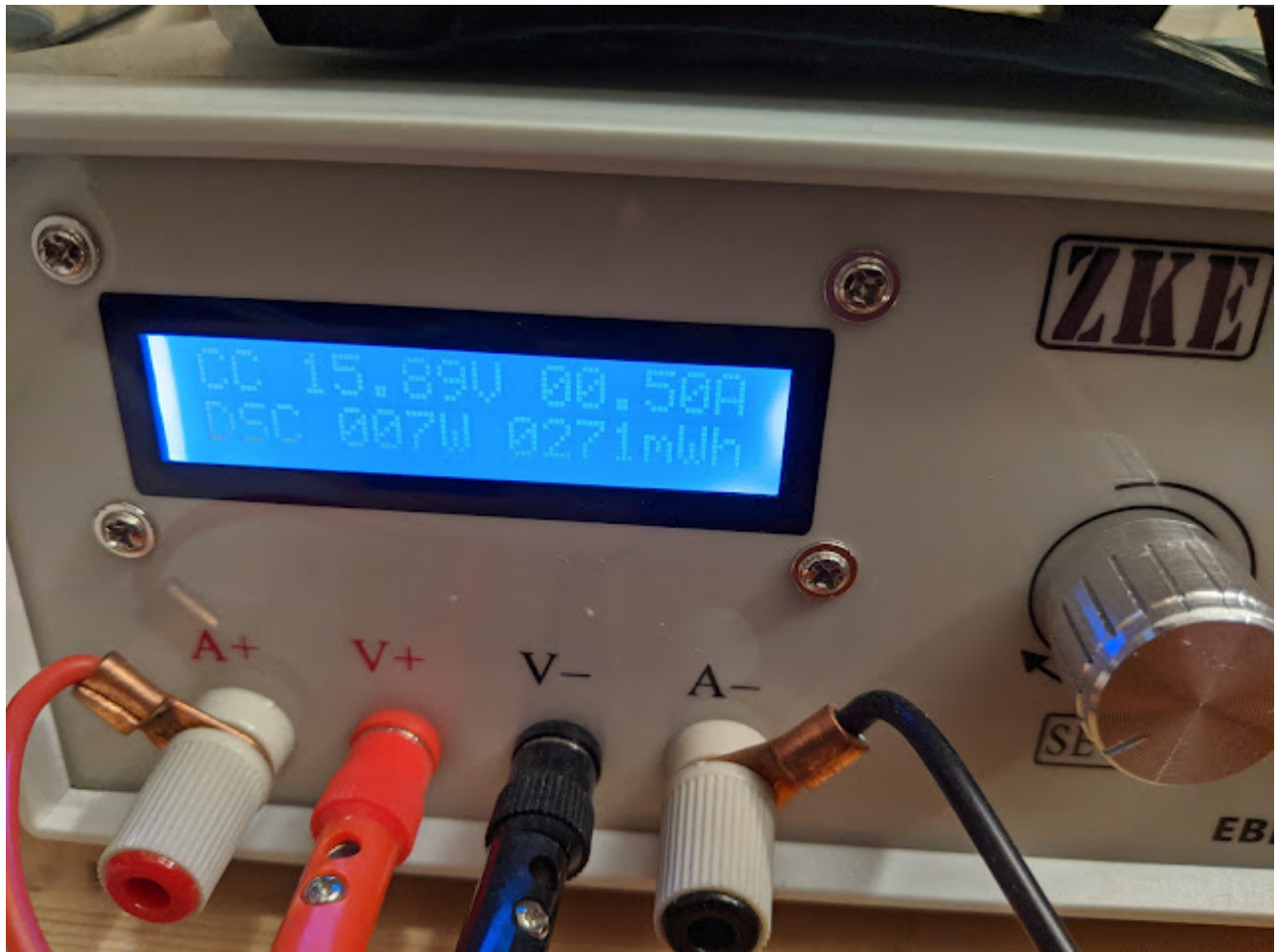
0.5 Amp test load on the +16vdc line.
