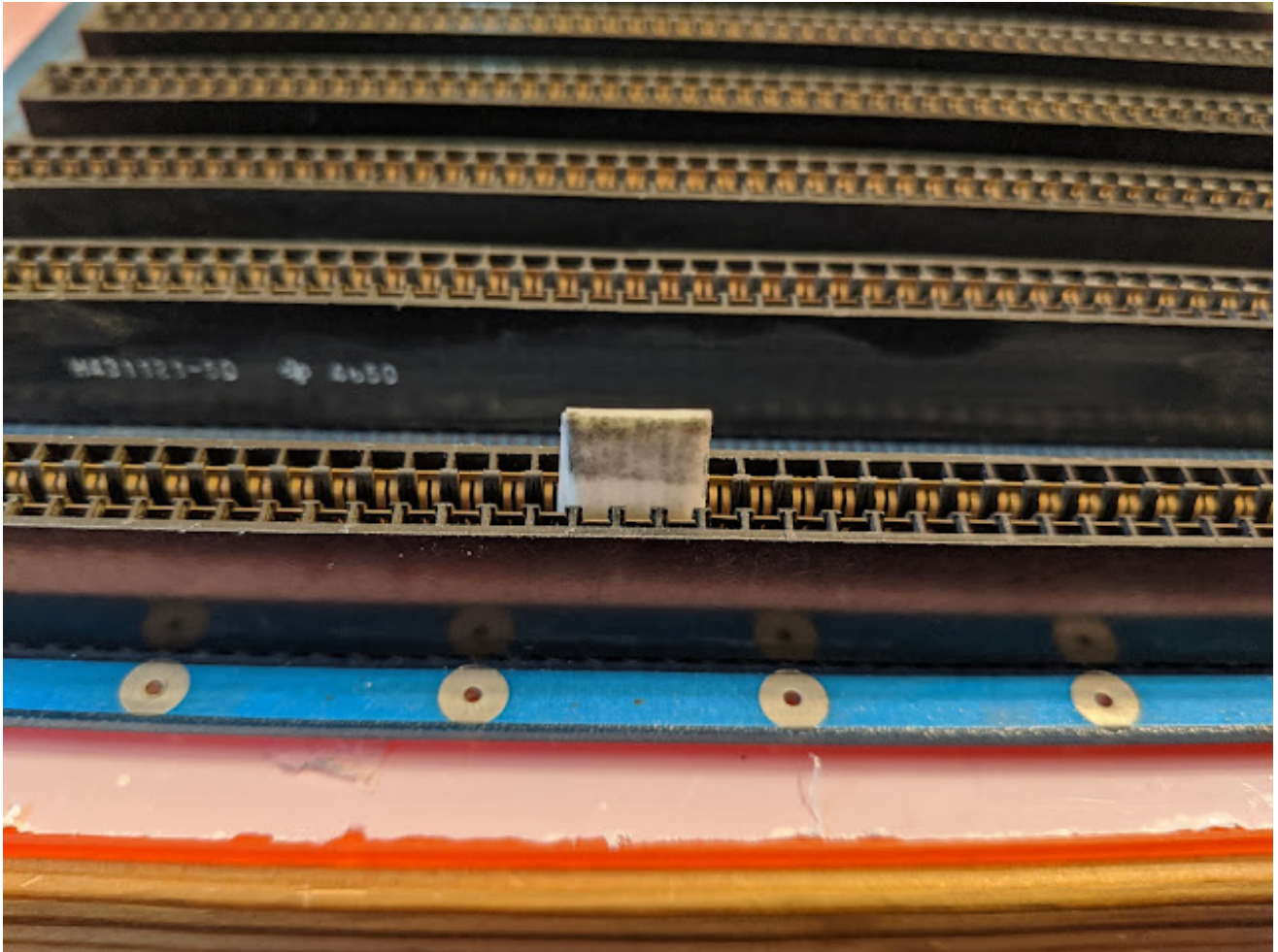
Cleaner Strip folded to 4 layers thick. It is now about 2cm long.
