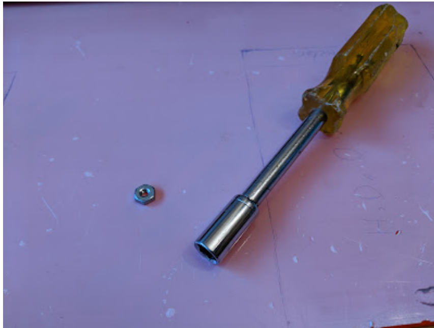
An invaluable tool for removing and refitting the Backplane nuts
