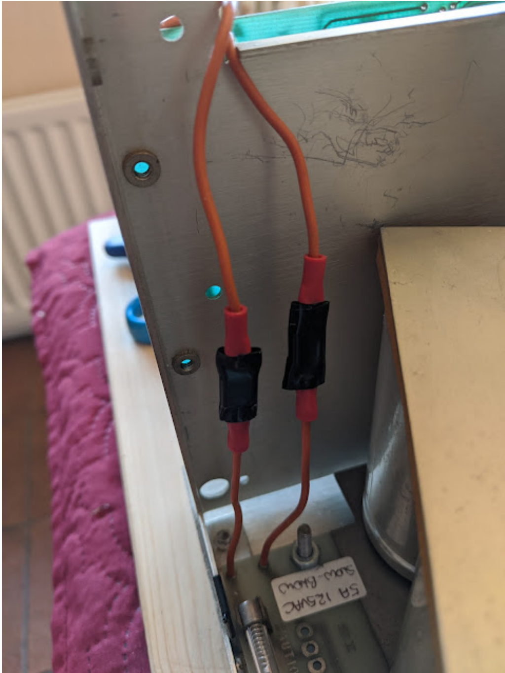
Mains supply to ON/OFF switch cut and crimped.
