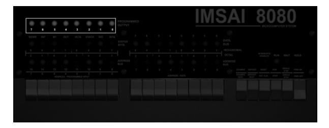
The LEDs are under software control. When a value is sent to I/O Port 255, the inverse binary number is displayed. For example, sending 0 to OUT 255 will turn all LEDs on, and sending 255 to OUT 255 will turn them all off. The CMP A instruction is useful, as it will quickly invert the value of register A, making the output more natural.
