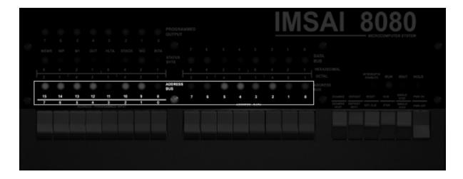
When the computer is not running, the WAIT light is on, and EXAMINE or EXAMINE NEXT, or DEPOSIT or DEPOSIT NEXT, or RESET has been toggled, these LEDs represent the current address.
