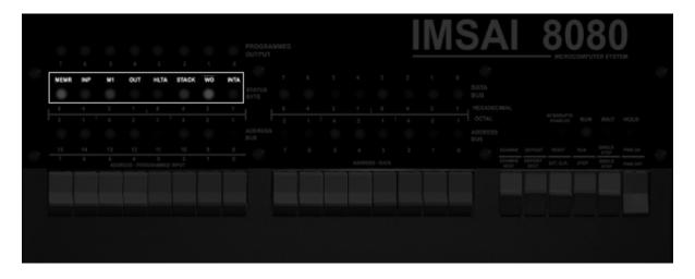
These LEDs give you a very low-level glimpse into what the CPU inside the computer is actually doing. You rarely need to use these unless you are debugging machine code.
