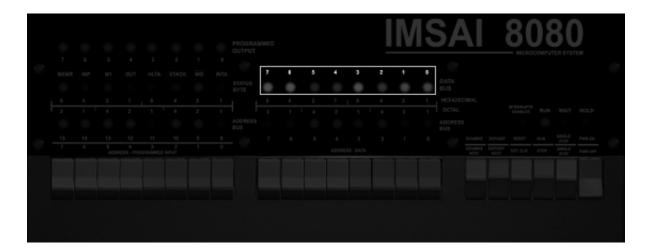
When the computer is not running, the WAIT light is on, and EXAMINE or EXAMINE NEXT has been toggled, these LEDs represent the data stored at the current address.
